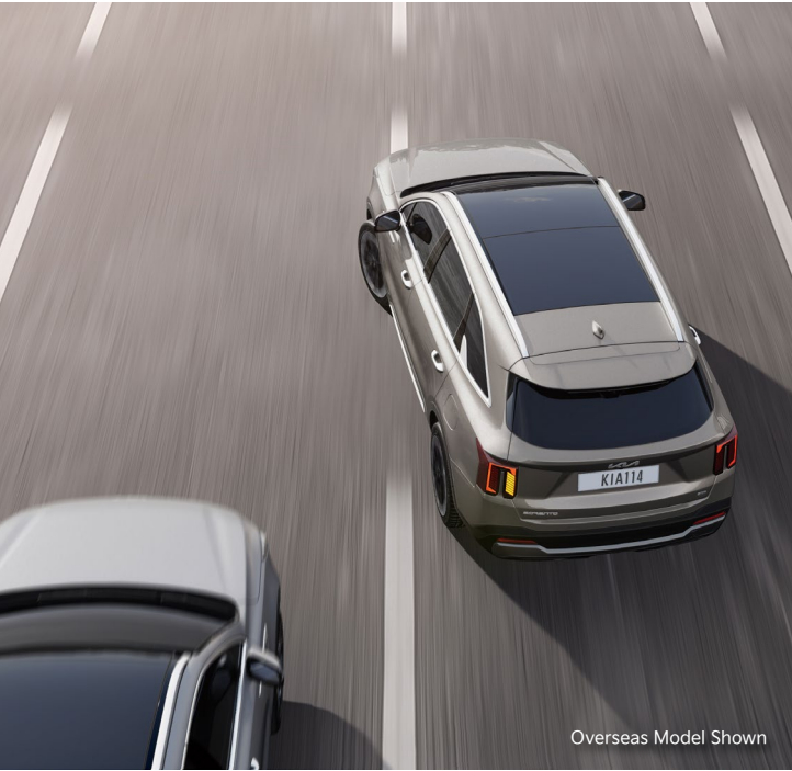
Blind spot Collision Avoidance Assist warns you if there is a risk of collision with a rear side vehicle in the blind spot while changing lanes.
